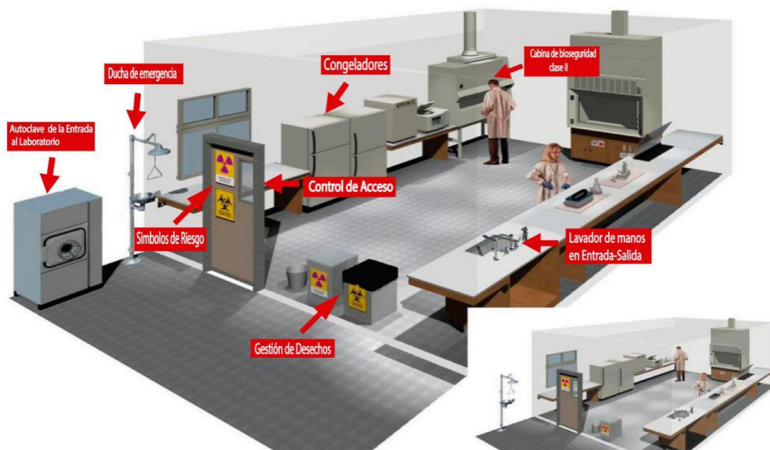
Figura 3. Laboratorio de Bioseguridad Nivel 2. Fuente: Laboratory biosafety manual Third edition-World Health Organization, Geneva, 2004.
